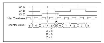
Figure 7-18. Channel Z Reload with X4 Decoding
